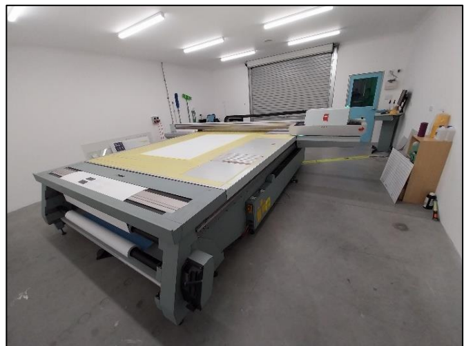
Printed Splashbacks produced in house on a Canon Arizona 1280XT – Digital UV Flatbed Printer. Capacity 2500mm x 3080mm
